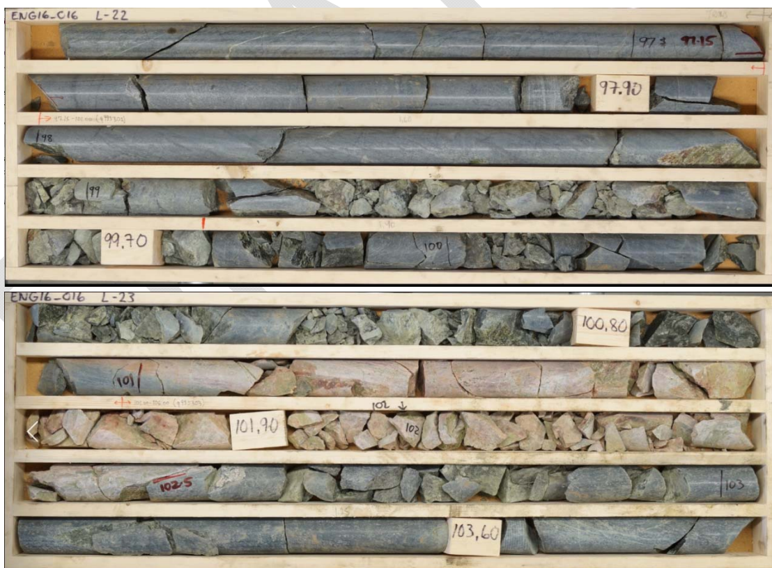
Figure 5-7: Significant fault logged in ENG16-016
