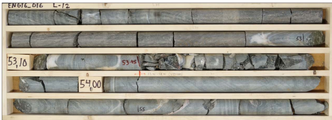
Figure 5-6: Minor fault typical of most broken intervals: fracture zone intersecting core at very low-angle; negligible fault rock
