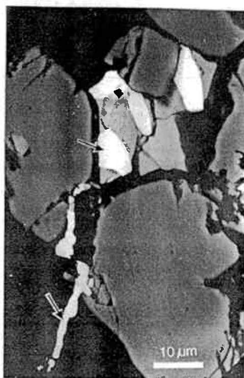
FIG. 24. SEM back-scatter picture of Cu-Au-Pd alloy (white), Fe-Ni sulphide (light grey) and chromite (grey).
