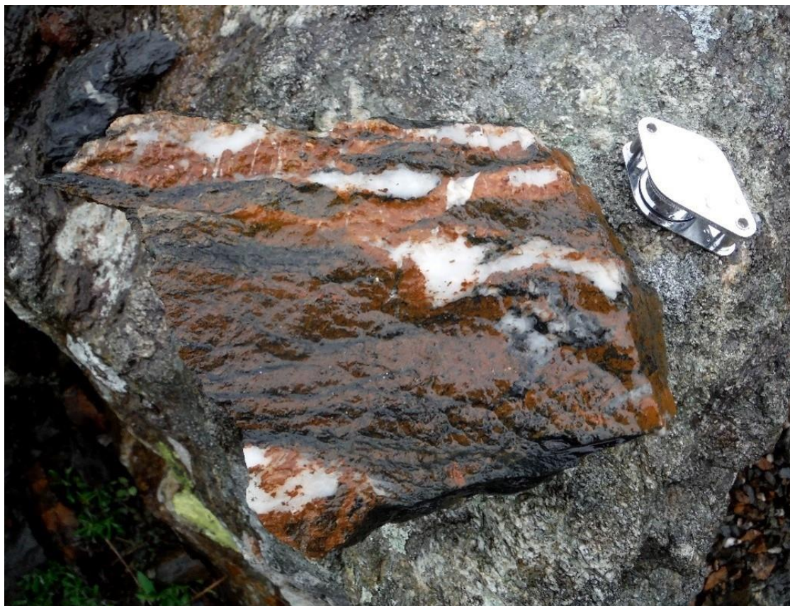
Figure 2-7: Fragment of quartz vein material from Oscarsgangen showing ribbons of host rock, abundant ankerite and disseminated pyrite
