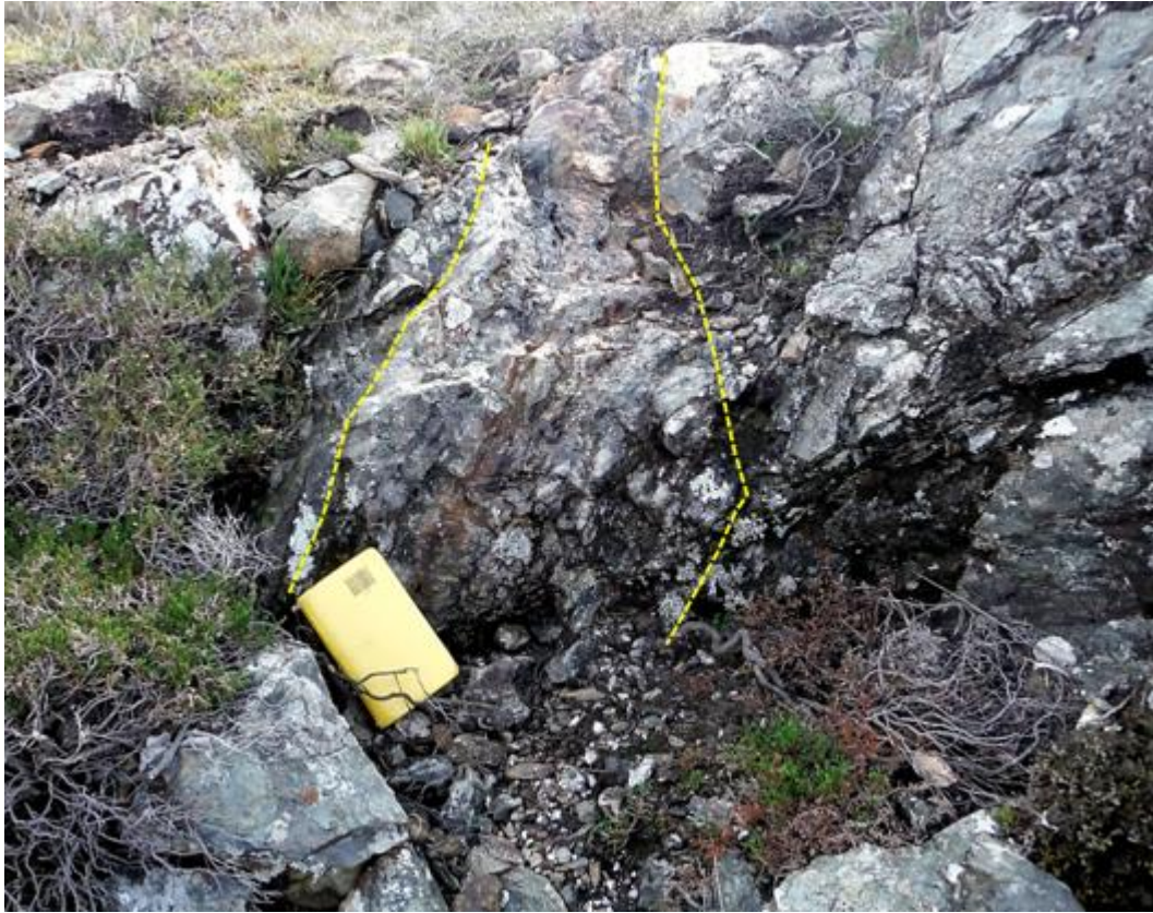
Figure 2-8: Outcrop of gold-mineralised quartz-sulphide vein in sheared gabbros in the southern part of the licence
