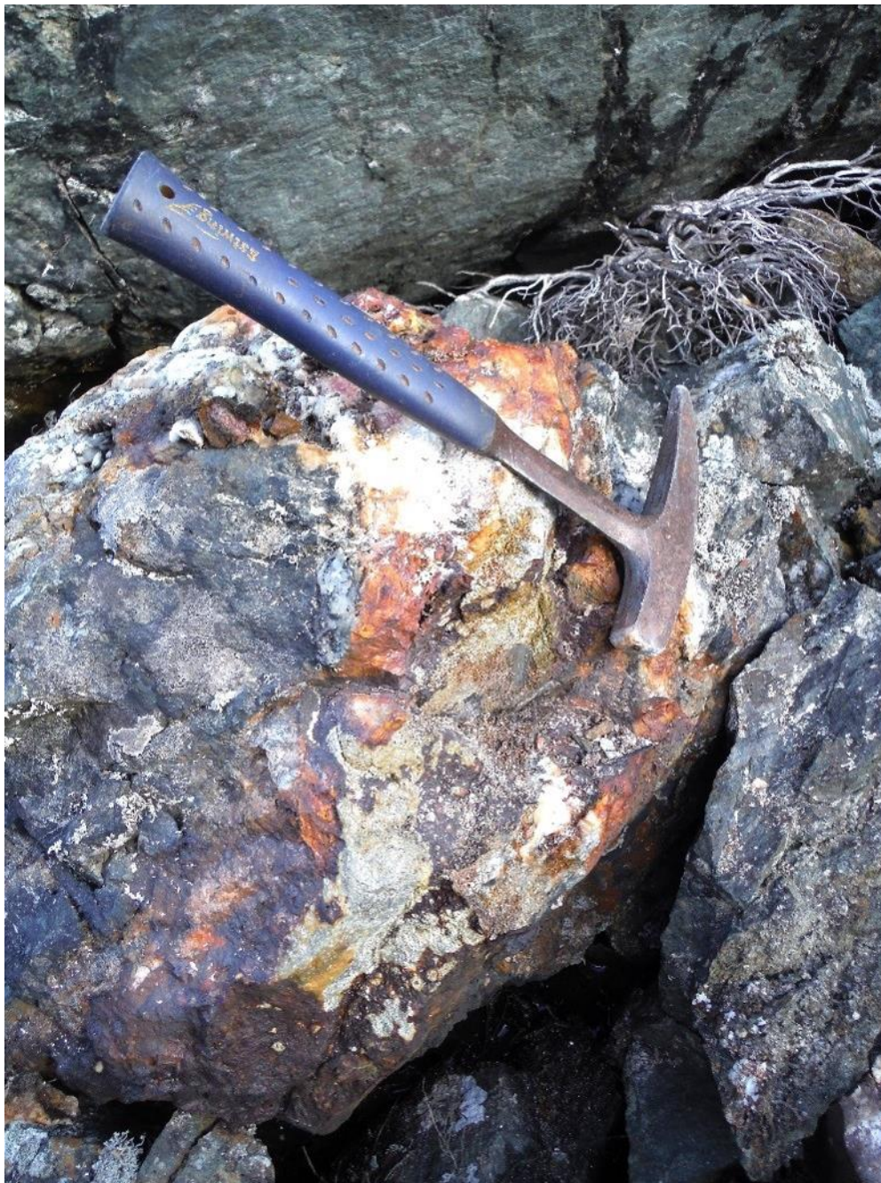
Figure 2-9: Boulder of quartz veining with abundant pyrite and chalcopyrite at the same location as in Figure 2-8
