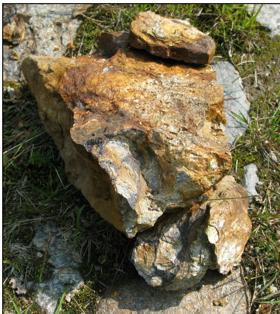
Figure 4.0.G: The largest of the two ore specimens found embedded in the gravel road at the roadcut. The lower fragment was cut and polished and is also shown on the front page of this report.
