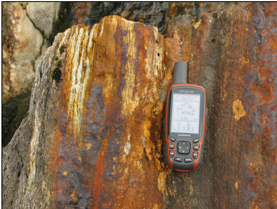
Figure 4.0.I: A close-up of the rust zone at Tjo7. Sericitic alteration with weak dissemination of fine-grained pyrite. At the GPS's antenna is a slightly more weathered zone that could very well be 1-2 cm of massive sulphide.
