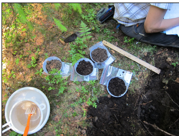
Figure 4. Equipment used for MMI sampling.
