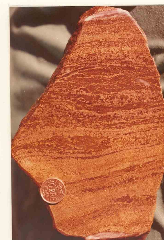
Plate 47 : (local. Vifte 43A nr.3) Banded magnetite and quartz-rich pyritic ore. Shows intense tectonic banding. Note, minor white carbonate bands, top and bottom.
