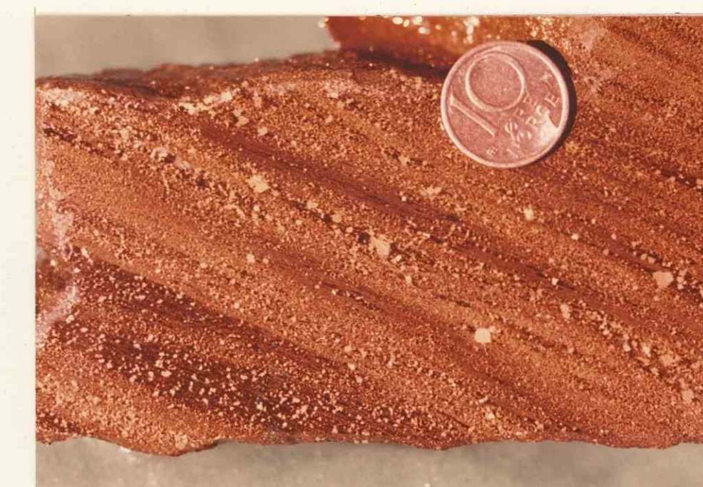
Plate 51 : (local. Fl.O. 160 nr. 12) Sedimentary pyrite - disseminated ore : well-banded, schistose, chlorite rich tuffs (dark), carbonate, and minor sphalerite rich, fine-grained pyrite (light). Note large well formed pyrite cubic porphyroblasts in dark chloritic schist bands, and extremely fine pyrite dusting in the dark chloritic bands.
