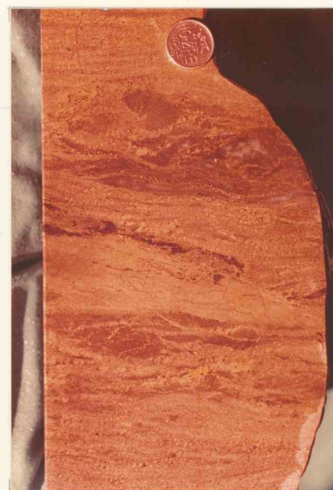
Plate 45 : AR 14 (R300/K.O.7 nr.6) Tectonically banded and minor folded massive Cu-rich pyritic ore. Note, much lensoid, dark-grey siliceous material and minor black magnetite bands. Hint of F_2 crenulation style minor folds.
