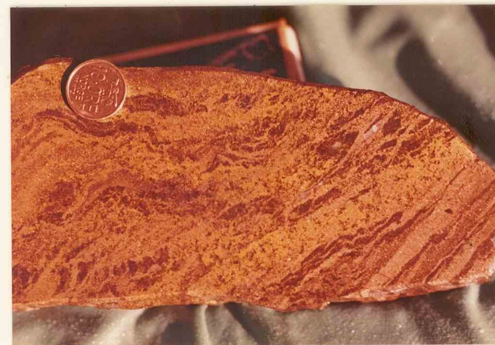
Plate 46 : (local. I.F. 13V/76 profile) Well-banded (primary) magnetite (black) and Cu-rich massive pyritic ore. Shows F_2 style minor fold structures.
