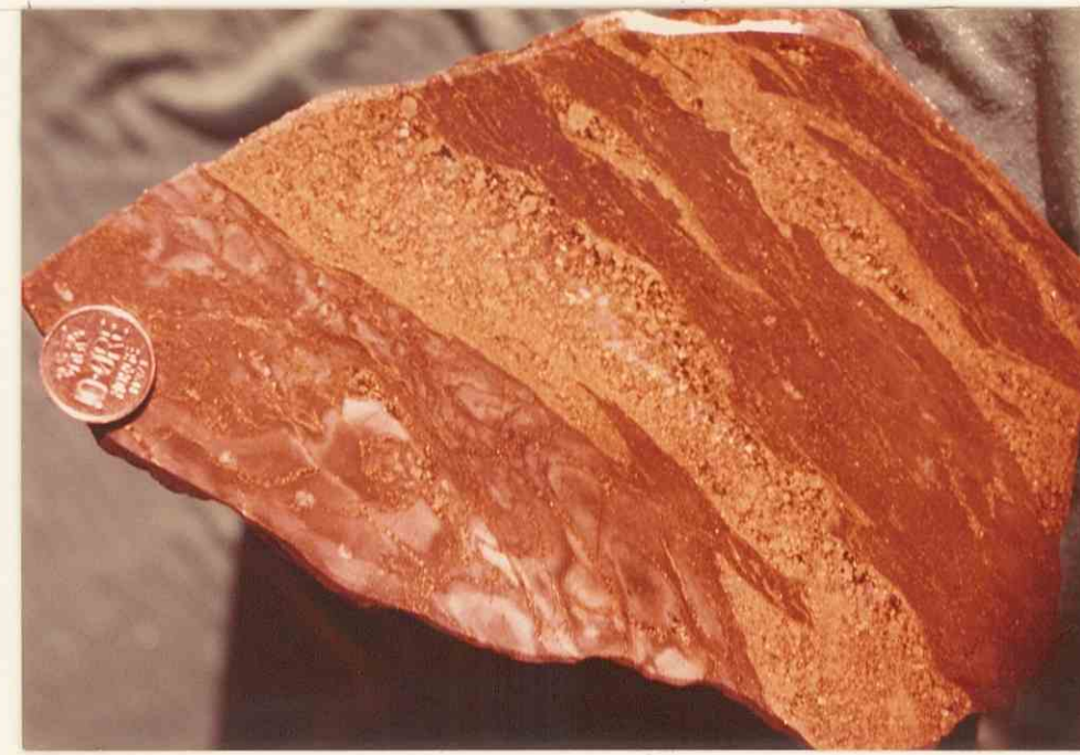
Plate 42 : (local. I.F. W4- 8V/778/685) Keratophyre - white felsic Rhyo-dacite : Appears to be white zoned fragments of hydrothermal alteration material similar to that associated with sulphide veining in plate nr. 40. Dark greyish material reflects very finely disseminated sulphides (pyrite?).
