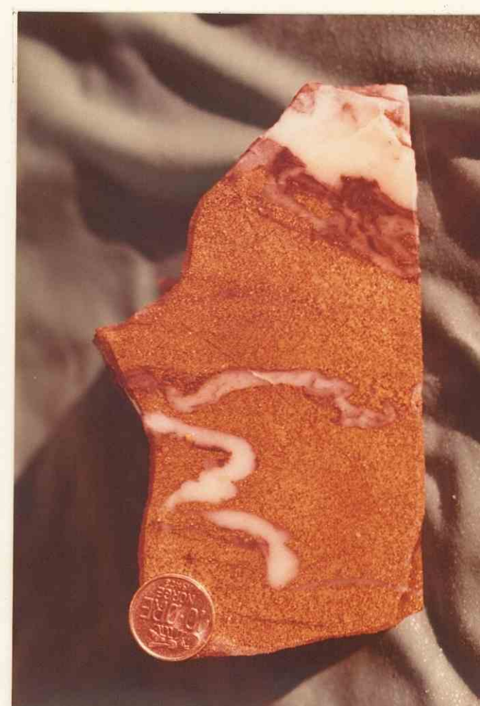
Plate 49 : (local. Vifte 43A nr.3) Carbonate banded, massive pyritic ore at locality near magnetite-banded ore (Plate 47). Note, coarser grain size of the massive pyrite with carbonate matrix, and isolated minor folding in carbonate band (white).
