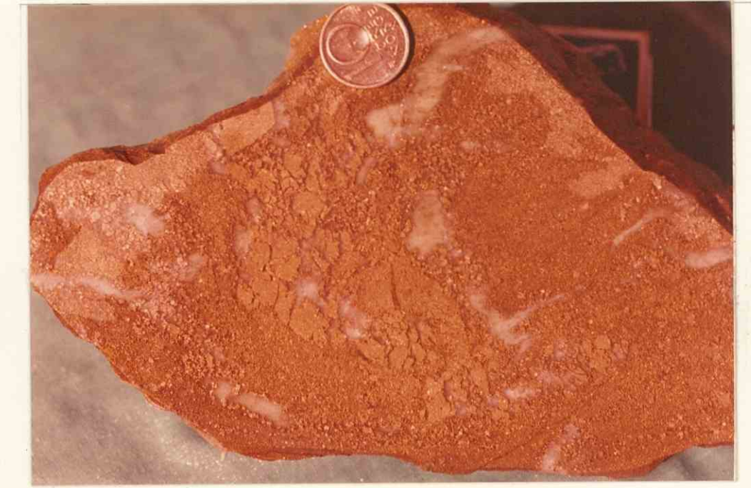
Plate 44 : (local. V.St.O. 10V nr. 10) Massive, brecciated, and coarse-grained porphyroblastic pyritic ore, with infolded and broken acid (quartz and albite) volcanic material, which probably represents acid volcanic veining.
