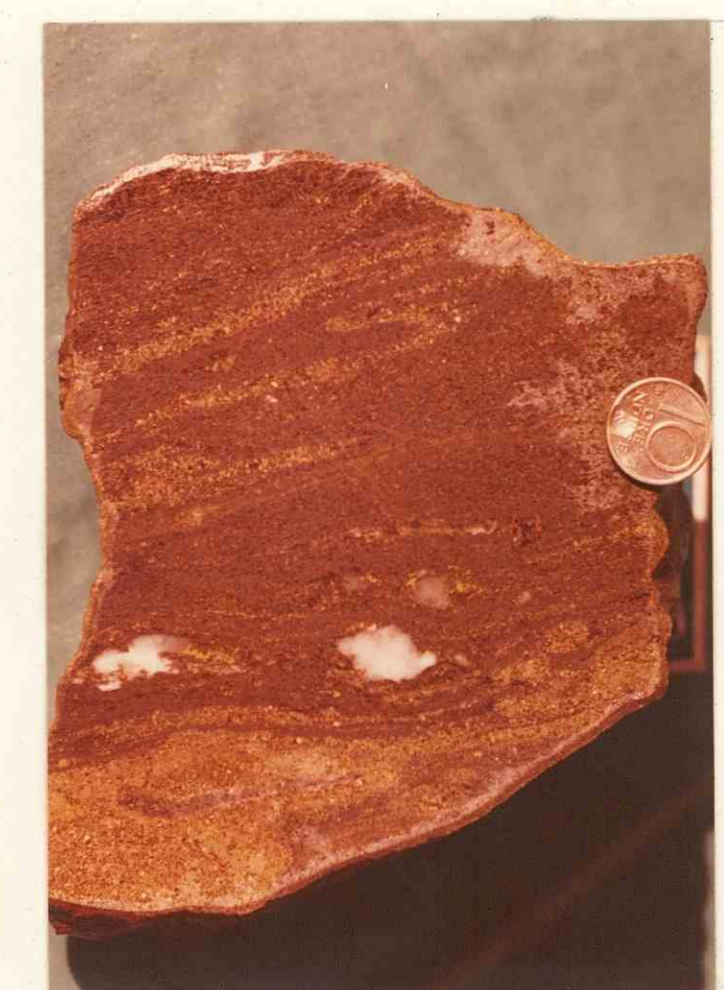
Plate 52 : (local. B.O. 320 nr.4) Massive sphalerite rich peripheral ore band, with minor folded pyrite rich bands (light color), and numerous white to clear quartz inclusions. Pyrite band at lower contact.
