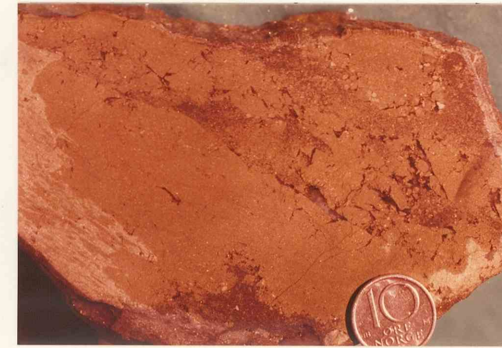
Plate 43 : (local. Sk.O. 50 e ) Typical S-rich Skorovas pyritic ore, extremely fine-grained, and compact. Shows clear quartz in matrix and as fracture fillings, and dark sphalerite concentrated at lower contact.
