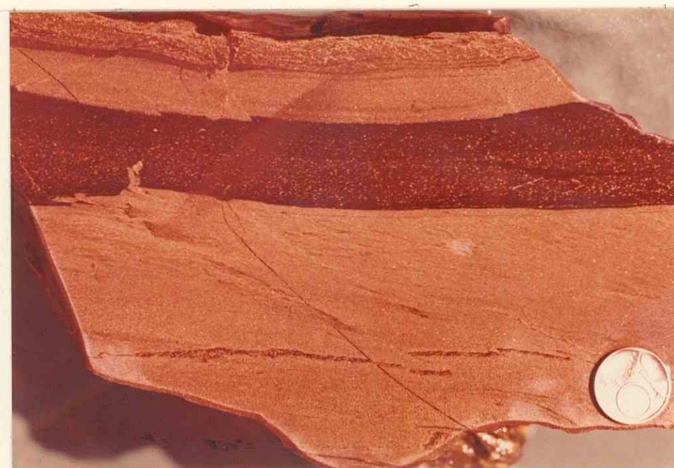
Plate 54: Typical well-banded, distal exhalite(vasskis) band from Tredjevatn area south from Skorovas.
