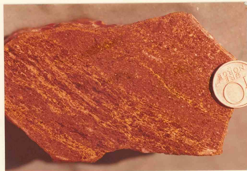
Plate 53: (local. B.O. 320 nr. 4) Tectonically banded, extremely schistose, massive Zn - Cu - Pb peripheral ore. Greyish material, massive sphalerite, light bands composed of chalcopyrite and galena, and dark colored minerals are amphibole needles, probably an Fe rich amphibole (grunnerite?).
