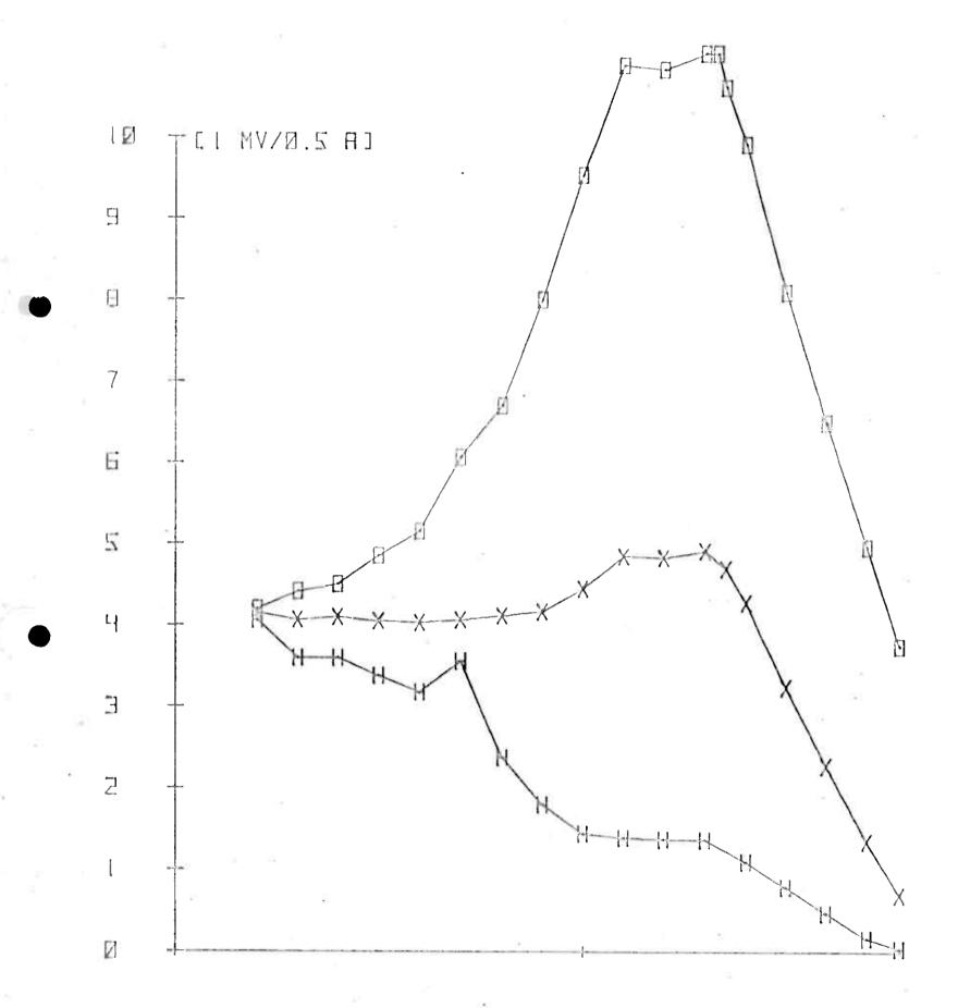
CHARGED POTENTIAL PROFILE BLEIKVASSLI / APRIL 1975 SCALE I TO SØØ BOREHOLE 3ØA
