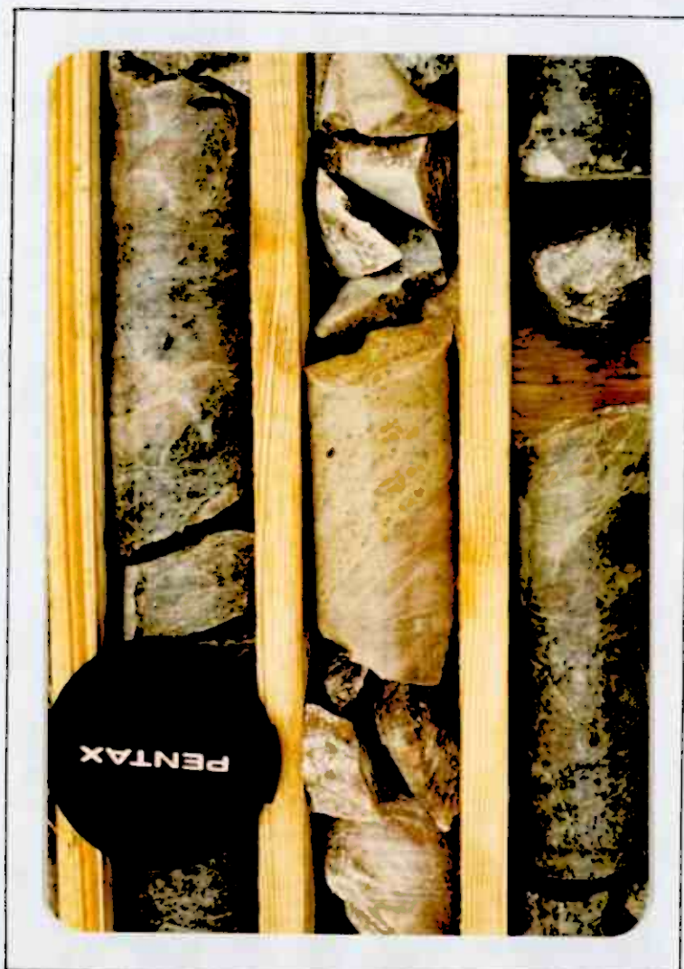
Photograph 21: Brecciated epidotised/albitised material in borehole 1 at approximately 80m.
