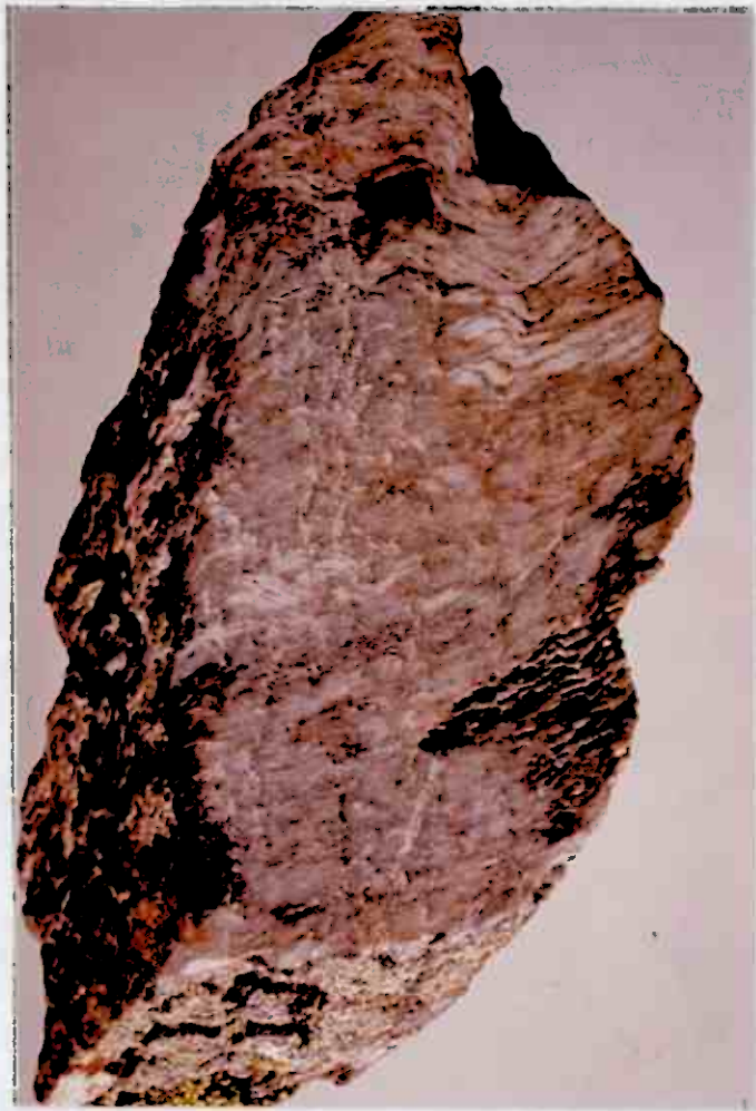
Photograph 27: Slabbed specimen of RH 139, showing possible primary chert laminations.
