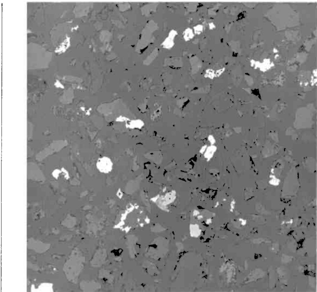
Same sample as given in Figure 3, except at higher magnification to show that most of the iron oxides (white) are interlocked with the celsian and other low reflecting minerals.
