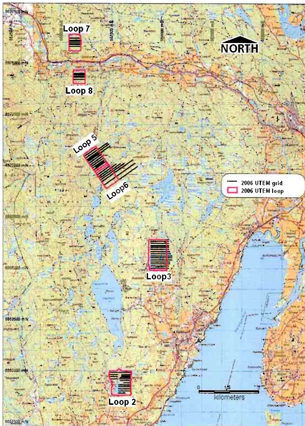
Figure 7 Ertelien Project: Ringerike Kommune – 2006 UTEM Grids and Loops
