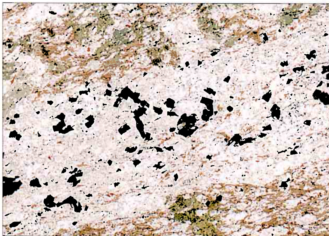
Figure 6 Microphoto showing colourless quartz, off-white plagioclase and calcite, brown biotite, light green amphibole, fine-grained ilmenite (black rectangular) and pyrrhotite (black irregular but // foliation), and coarse-grained (black) arsenopyrite. Field of ca 1.5 cm, one nicol.
