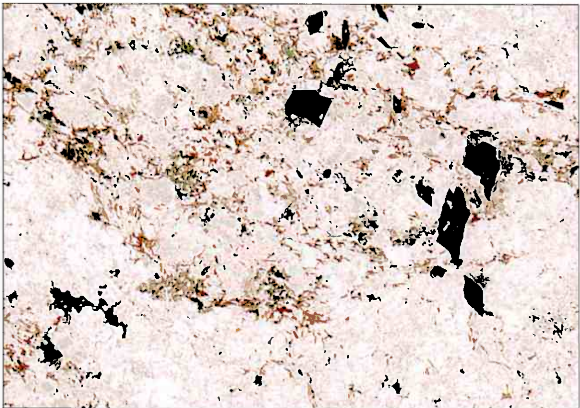
Figure 9 Microphoto showing colourless quartz, off-white plagioclase and calcite, brown biotite, light green amphibole, fine-grained ilmenite (black rectangular) and pyrrhotite (black irregular but // foliation), and coarse-grained (black) arsenopyrite. Field of ca 1.5 cm, one nicol.
