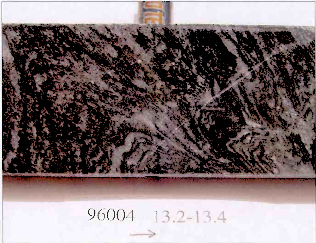
Fig 12. Very strong carbonatization is seen in the right part creating a “ghost structure” This destroys the dark minerals (biotite and amphibole) both chemically and mechanically almost completely. The dark bands seen in the right part mainly consist of ilmenite.
