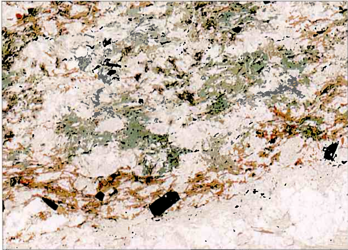
Figure 4 Microphoto showing colourless quartz, off-white plagioclase and calcite, brown biotite, light green amphibole, fine-grained ilmenite (black rectangular) and pyrrhotite (black irregular but // foliation), and coarse-grained (black) arsenopyrite. Field of ca 1.5 cm, one nicol.
