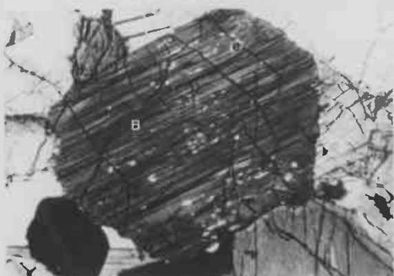
Plate 29 Chromite (c) enclosed in plagioclase (Iv 17). Field of view 3.6 mm
