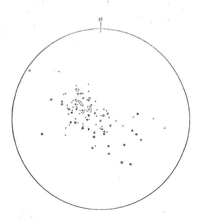
D1 stretching lineation. x - long axes of pebbles, o - slickensides, - fibre lineation in pelites.
