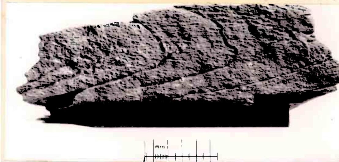
Fig. 13.17( below). Specimen 679. Showing aggregates of etc. & muscovite as in fig 13.16. Syn-schistosity fold.
