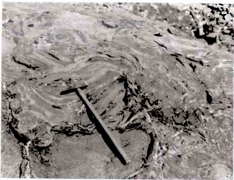
Fig. 4.2 Part of amphibolite mass within Furulund schist at Giken, (south of the road, west of the bridge). The rock is in an advanced state of brecciation.
