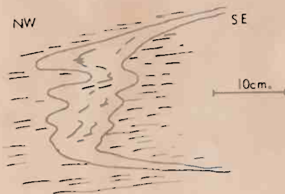
FIG. 5.7 Syn-schistosity fold of calcareous band in the Furulund schist. Photograph is taken almost along the fold axis. Location- about 1km. east of Giken.
