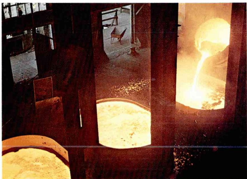
Discharging of the molten ferrosilicon.
