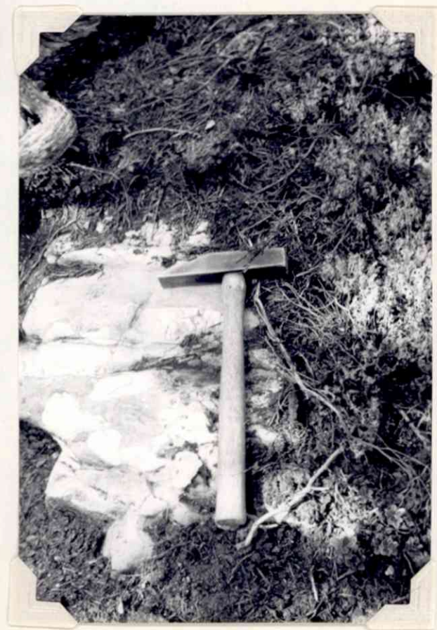
511 Another photograph of a very typical tuffaceous → conglomerate. Identical conglomerates occur also west of the Kavaa River and also west of the Bogo River. The white colour is due to the weathering of feldspar, reflecting the highly feldspathic nature of the rock. 450m. N.N.W. of Blomli
