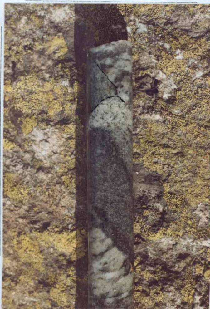
Iron sulfide mineralisation in banded gneiss, cut by two generations of aplites. DH 5B.
