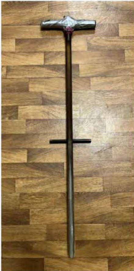
Photo 1: auger used for MEFFA sampling
