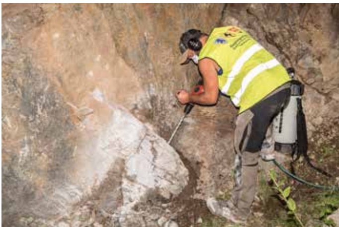
Figure 2.7 Surface samples, as little weathered as possible, has been collected using hand-drill, sledge-hammer, diamond chain-/circular saw or dynamite.
