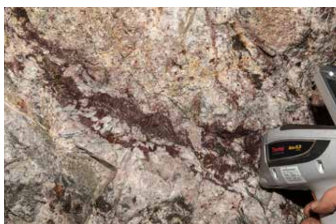
Figure 5.4.2e REE-mineralization in a vein in the FSS mine. The massive red-brown zone contains > 16 % REE (La+Ce+Pr+Nd measured by handheld XRF as elements).
