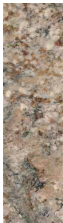
Figure 7.2.3e LHKB-2 633.2-633.7m FDC with REE-mineral aggregates (yellowish brown)
