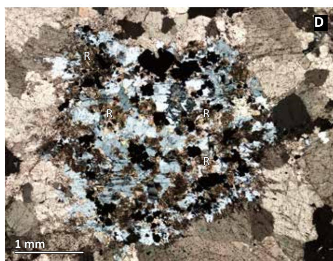
D. The REE-bearing domain in C in optical microscope. PM-TL-XP. The domain consists of a light mineral, mainly Brt. The REE minerals appear as tiny grains with high interference colors (some examples shown with R) in a matrix with various shades of gray. Opaque grains are magnetite. This domain, which is rather typical of the REE-bearing domains of this mineralization, has been studied in some detail in SEM-EDX.
