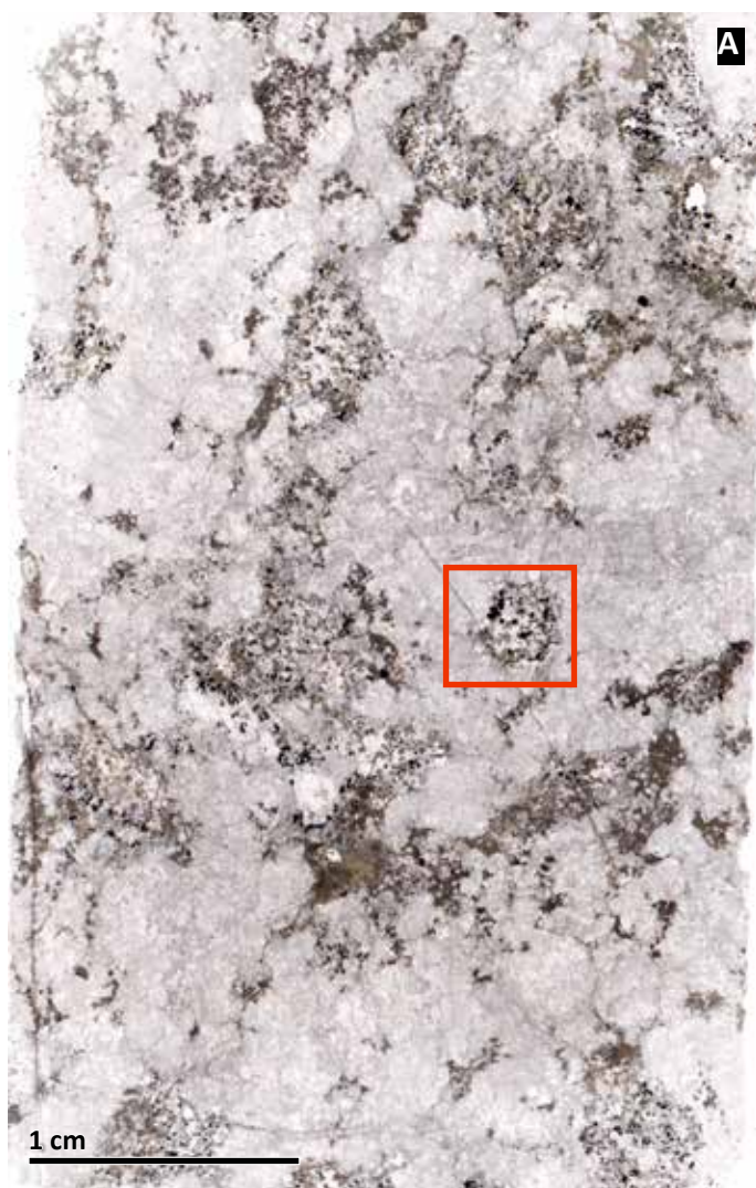
A. Scanned image of a thin-section. REE-bearing domains appear as rounded or irregular "dotted" areas. TL. Red rectangle shows the position of the image in figure C
