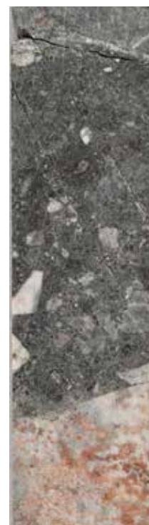
Figure 7.2.3f LHKB-2 408.5-408.7m REE-FDC-fragment (bottom) in damtjernite breccia (top).
