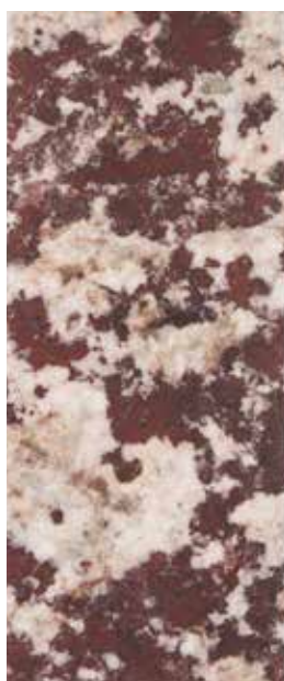
Figure 10.2.1 Hematitized REE mineral aggregates from drill-core (35 mm wide).
