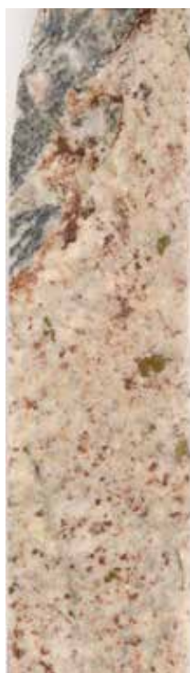
Figure 7.2.3c LHKB-1 101.0-101.2m Granular REE-FDC. REE's occur in the red aggregates.
