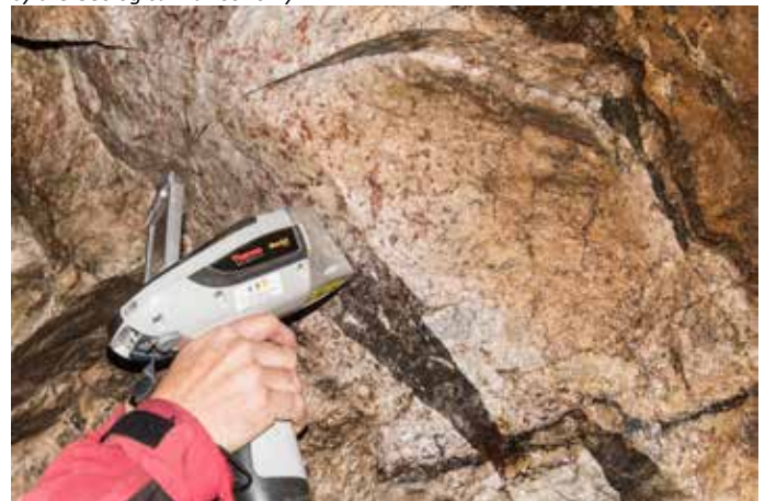
Figure 2.8 Extensive use of a hand-held XRF (records La, Ce, Pr, Nd), and a hand-held gamma-spectrometer (U, Th, K), has been very important during the mapping.
