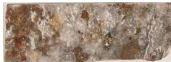
Figure 5.4.1c Drill-core T17, interval, from surface drilling at Tuft drilled by Norsk Bergverk. The red-brown aggregates are REE minerals. The core is 22mm wide.
