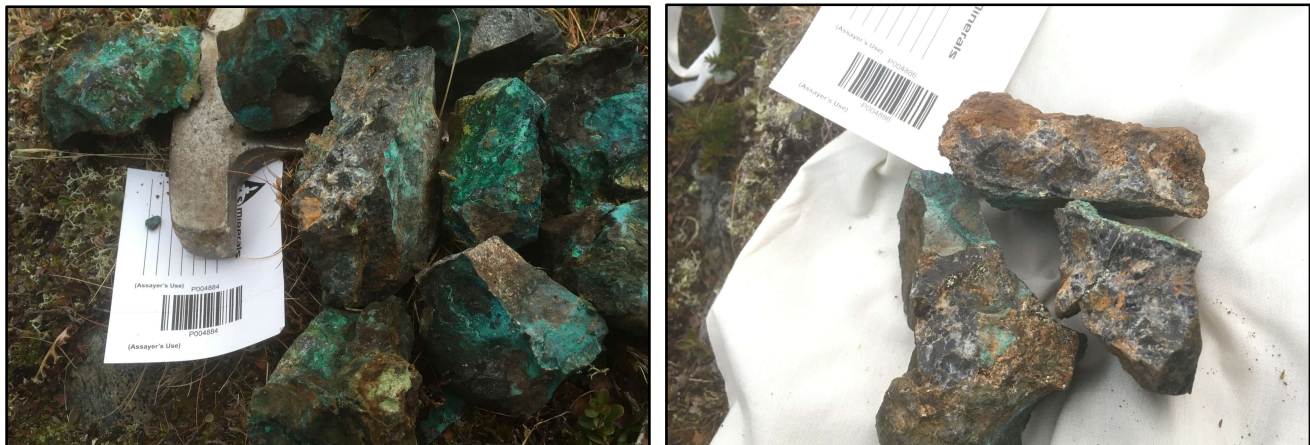
Figure 5 - Right: sample P004884 showing extensive secondary Cu staining in black silica. Left: sample P004886 showing chalcopyrite, secondary Cu mineralisation and FeOx staining in brecciated silica.
