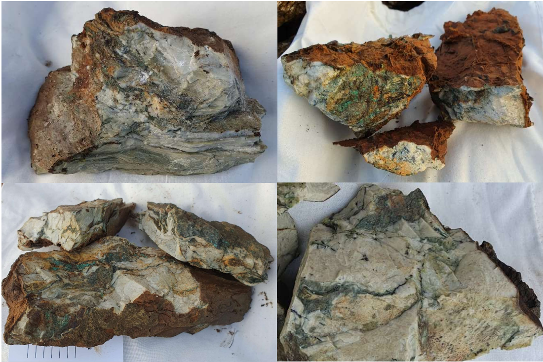
Figure 9 – Number of samples demonstrating the black ‘whisps’ within dolomite which contains bornite, chalcopyrite and chalcocite. With localised significant secondary malachite enrichment. Natural weathering of the dolomite is a strong orange brown with fresh surface much cleaner. Some samples show evidence of cross cutting smaller scale silica veins.
