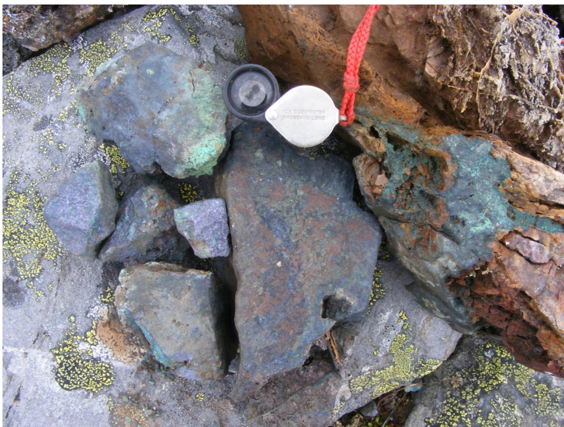
Fig. 26. Floats of massive bornite and chalcocite. UTM 554584 7747036.
