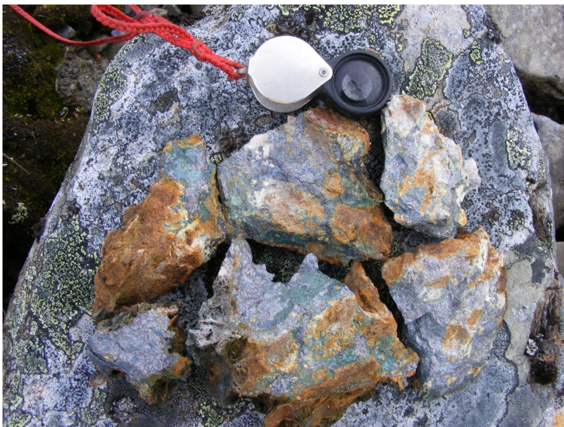
Fig. 28. Vein material of bornite mineralisation. UTM 554793 7747014.
