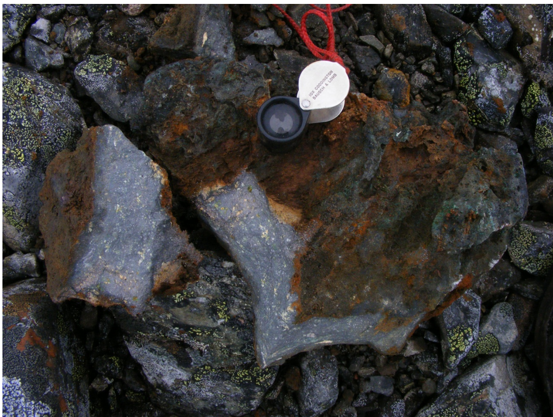
Fig. 27. 3 kg boulder of semimassive bornite and chalcosite at 554718 7746914.
